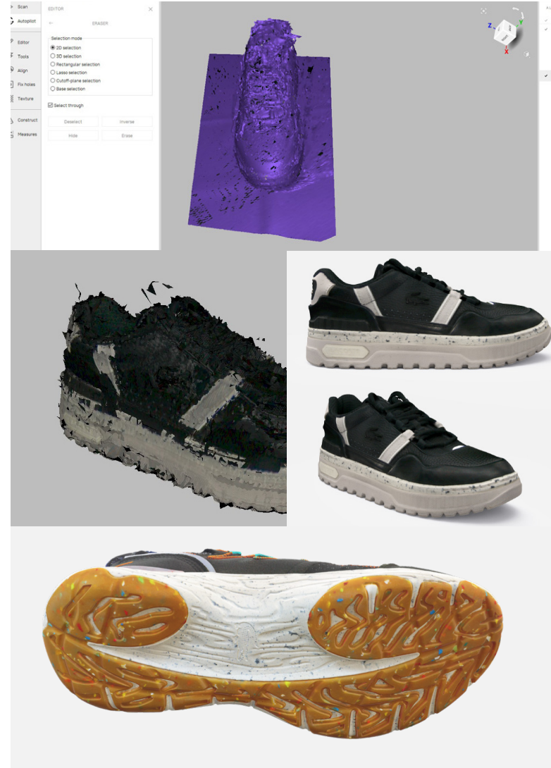
3D Scanning using Artec EVA scanner, utilised for reverse engineering archive styles & modelling existing models.
